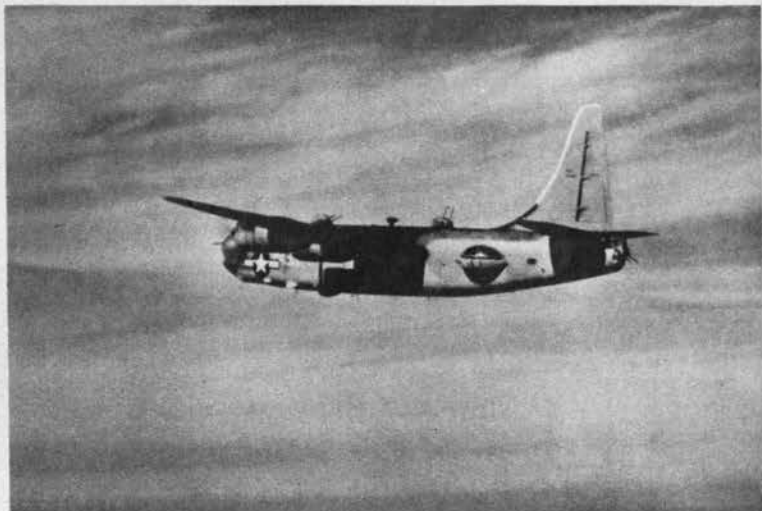
Navy Privateer , scanning sea around Marianas, is easily recognized by lofty single tail, waist blisters fitted to the familiar bulky B-24 fuselage.
